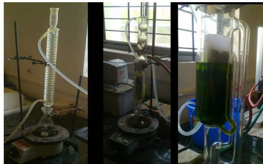
Fig 5. Heat reflux extraction. Soxhlet extraction apparatus
