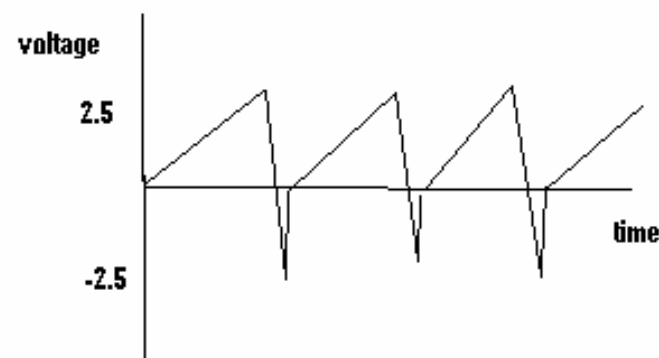
Figure 9: Typical signal from the MEMS sensor during seizure
